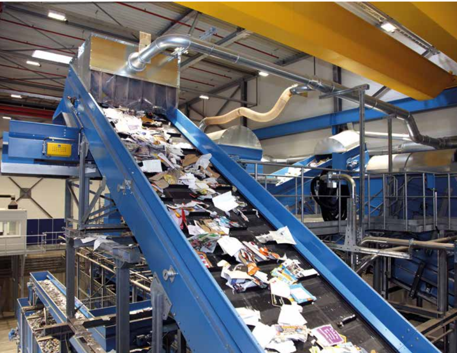
At Palm Paper in King's Lynn, the production of graphic papers is also based entirely on selected and sorted waste paper. Since 2019, a separate sorting plant for mixed paper has been in operation on the mill premises.
