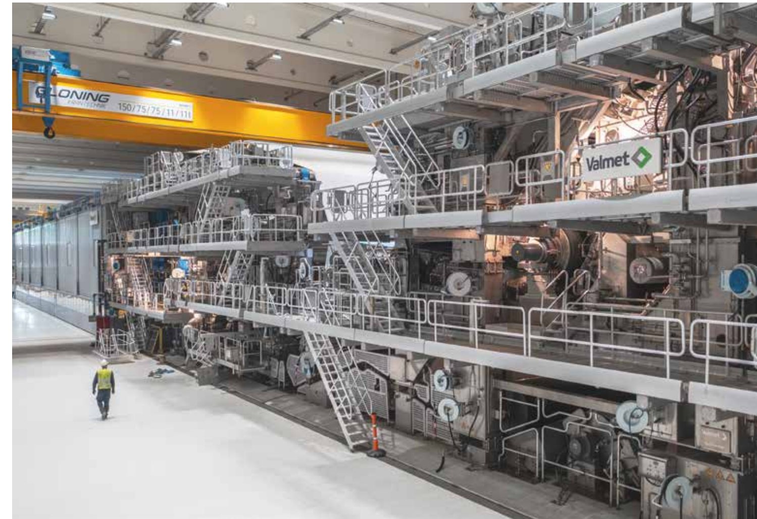
The new PM 5 in Aalen with a width of 10.90 m is specialised in the production of lightweight corrugated base paper.
