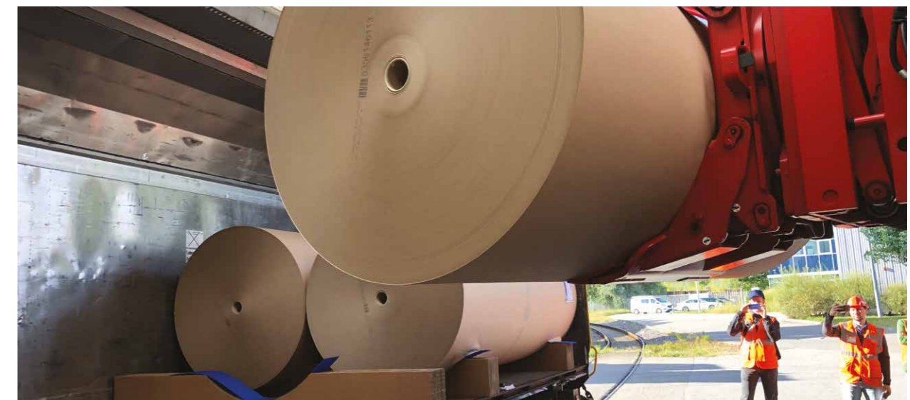
Sustainable load-securing device made of corrugated cardboard for transporting our paper rolls by rail.
